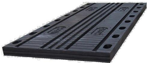
Agom AGFLEXJ expansion joints are designed to handle displacements of up to 330 mm between the bridge decks they are fastened to. Entirely waterproof, they are secured to the structure with suitable anchor bolts. The deformable rubber elements are vulcanised bonded with tough steel reinforcements (standard EN 10025). AGFLEXJ joints also allow displacement and rotation of the structure's parts relative to each other in any direction.
